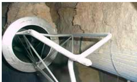
Horizontally mounted filter cartridges can cause dust to become entrained at the top of the filters, shortening filter life and providing a dusty surface for sparks to ignite.
