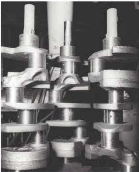
Fig. 1 — In the foreground are front sections of two crankshafts that have been coated. Between and behind them is a crankshaft yet to be repaired with scoring visible on the surface that will be restored by thermal spray.
