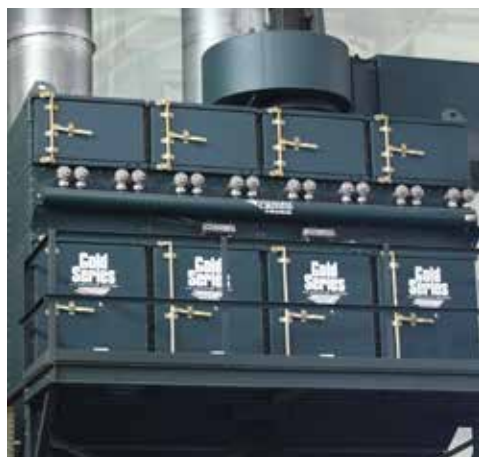
A safety monitoring filter system is integrated on top of the collector to enhance dust capture efficiency and provide backup protection. These filters are required before discharging exhaust air to the atmosphere when handling hazardous powders and metals such as nickel and chromium.
