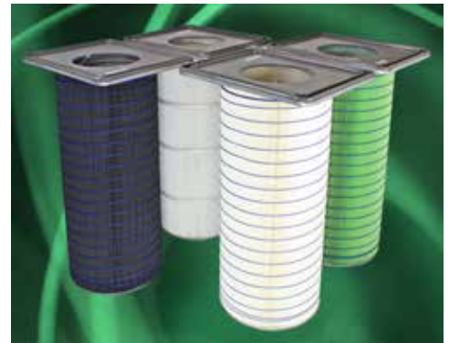
Filters with nano fiber media are recommended because the fine-pored nano fibers act as a pre-filter to the base media, capturing dust at the surface before it imbeds in the filter. This technology increases dust capture efficiency while enhancing cleaning ability and service life.
