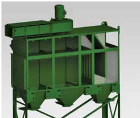
A drop-out module slows down the velocity of the air stream before it enters the dust collector. This can extend the life of the primary filters, reduce fire risks and aid in product reclamation.
