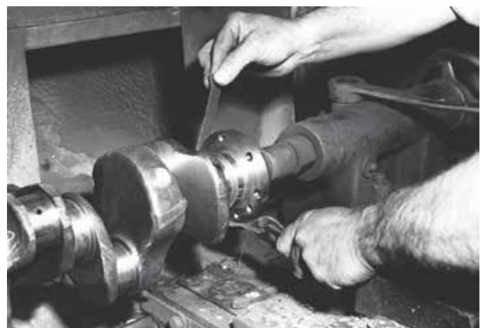
Fig. 2 — A Ford employee mechanically cleans the area to be coated by holding a coarse emery cloth against the rotating crankshaft that was previously solvent wiped.
