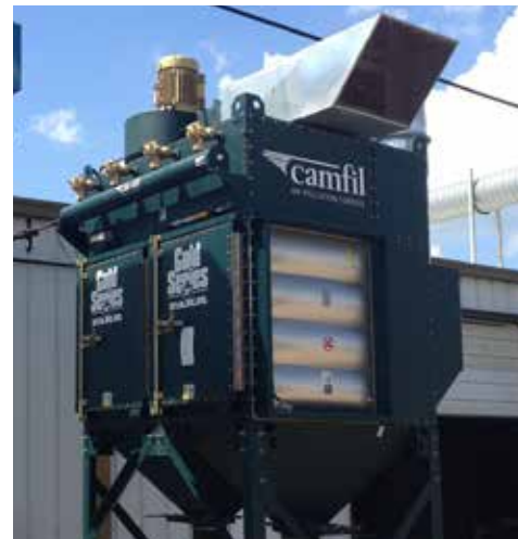
Used on a spray and fuse application, this dust collector has been in operation for nearly two years with no issues or maintenance needed. Benefits include low pressure drop for energy.
