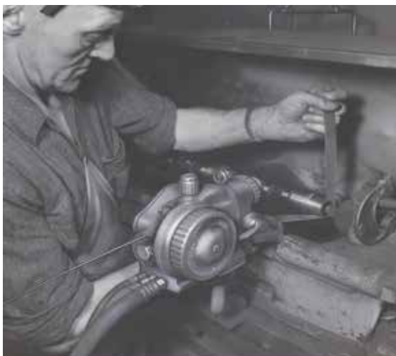
Fig. 3 — A Chevrolet employee mechanically cleans the area to be coated by holding a coarse emery cloth against the rotating camshaft.
