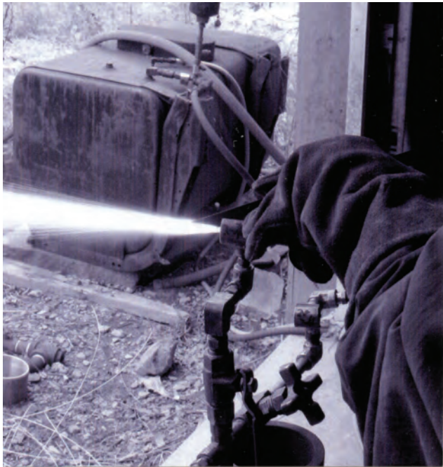
Figure 5. A 1/2 in. wide by 0.025 in. steel strip being sprayed by a V 1/8-3/4 burner using 500 scfh of Oxygen with a spray rate of about 20 lb/hr.
