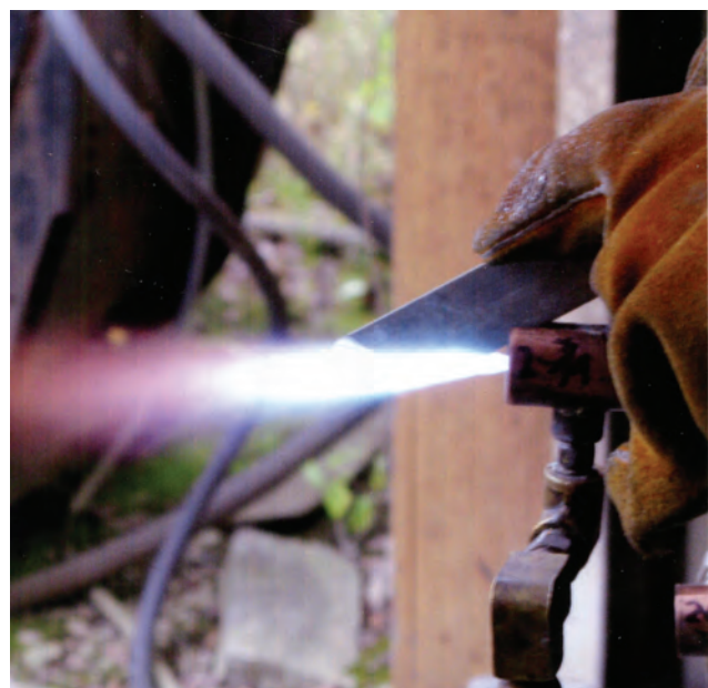
Figure 7. A 1 in. wide by 1/8 in. thick zinc strip using the V 1/8-3/4 burner — spray rate, “very high”.
