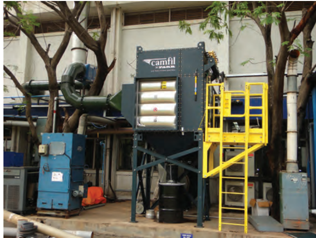
Gold Series GS6 dust collector for epoxy coating fumes/dust capture application.
