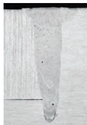
Crack-free EB weld in alloy 6061 alloy made using foil filler material.
