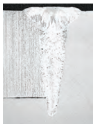
Crack-free EB weld in 6082 alloy made using cold sprayed buttering layer.
