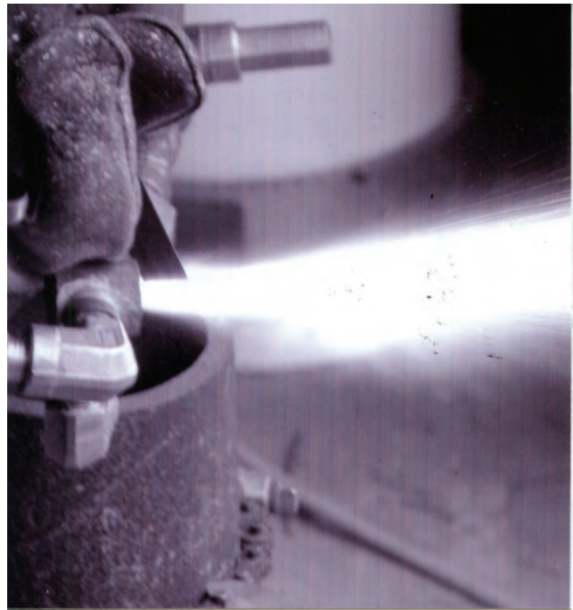
Figure 6. The wire strip of Fig. (5) being sprayed from a nearly vertical path into the jet from a 2V 3/8-3/4 spray gun at a spray rate of about 30 lb/hr using about 2,000 scfh of Oxygen.
