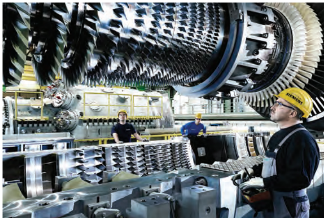
The picture shows the Siemens gas turbine SGT5-8000H during assembly in the Siemens gas turbine manufacturing facility in Berlin, Germany.
