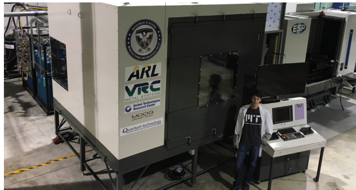
Fig. 4 — Cold spray helium recovery and manufacturing cell designed and demonstrated by ARL under the Defense Manufacturing Science and Technology (DMS&T) Program. More than 100 parts have been developed under the DMS&T.
