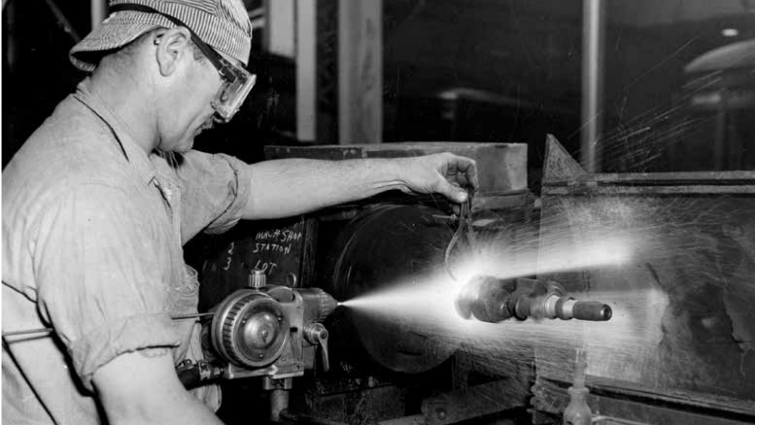
Fig. 4 — A worker oversees 0.25% carbon steel applied over an abrasive blasted crankshaft main bearing. (Note: In current safety practices, protective gear would have been worn.)
