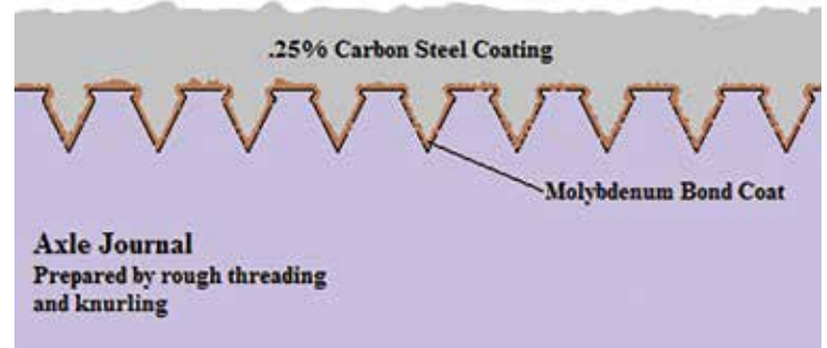
Fig. 1 — Molybdenum bond coat and 0.25% carbon steel applied over the threaded and knurled journal.
