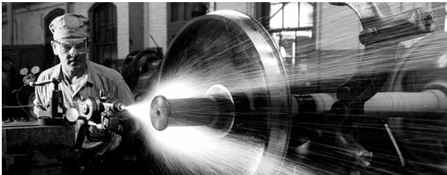
Fig. 2 — A New Orleans Public Transit employee oversees 0.25% carbon steel applied over the molybdenum-coated journal.
