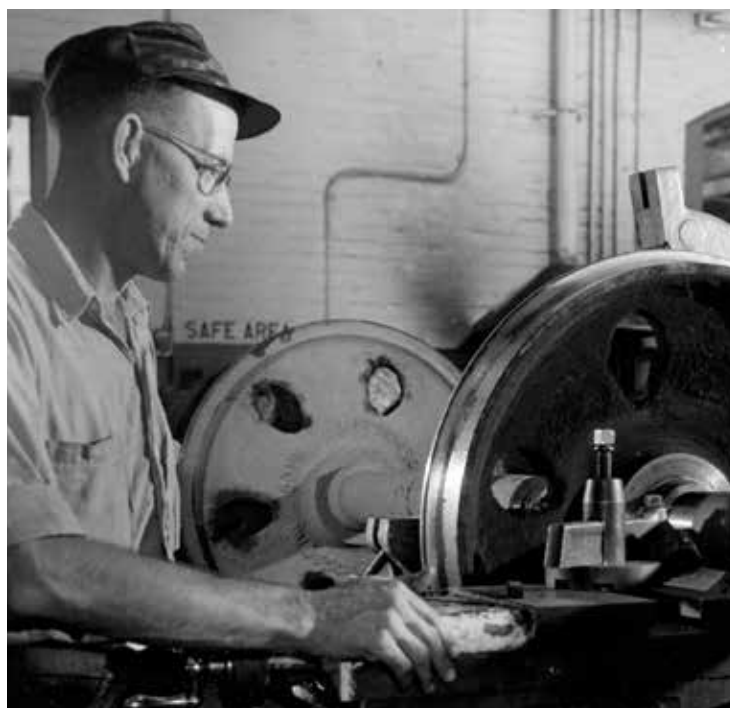
Fig. 3 — Thermal spray coated journal being machined back to size.
